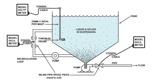
Markland's Suspended Solids Density Meter uses the attenuation of ultrasound to measure silt, sludge and slurry concentrations, and operates in the region between turbidity meters and nuclear gauges.
